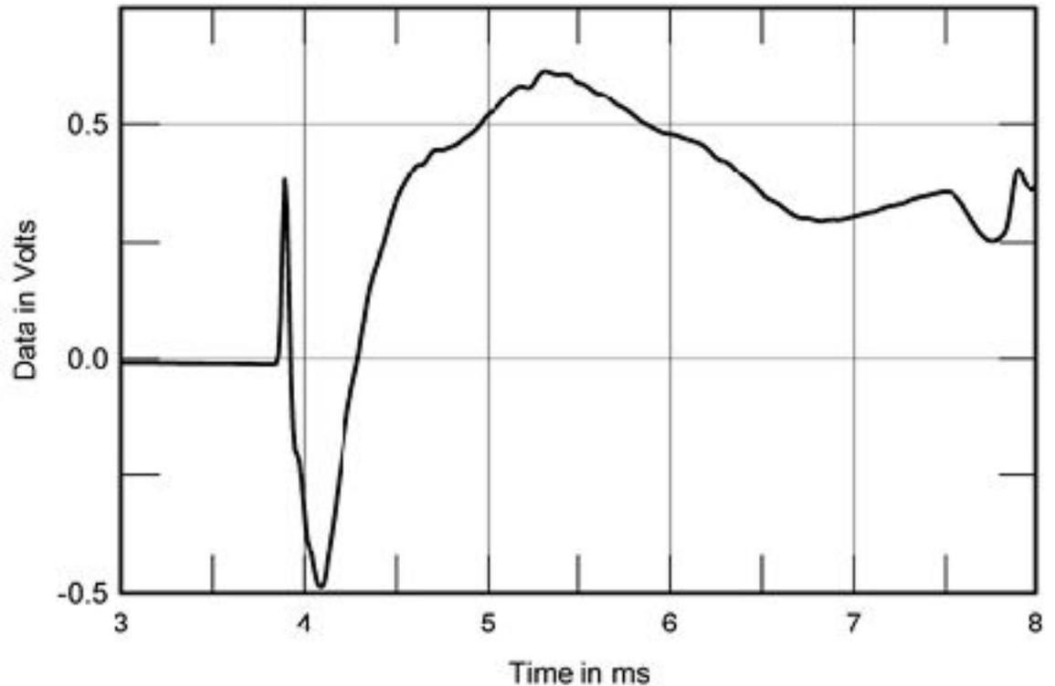
Fig.7 Mårten Design Coltrane, step response on tweeter axis at 50" (5ms time window, 30kHz bandwidth).
