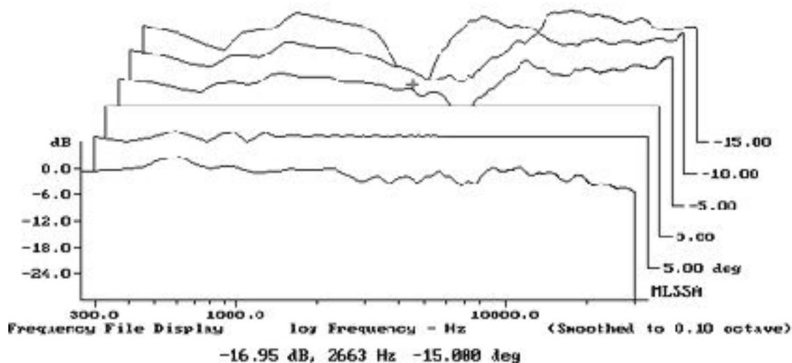
Fig.6 Mårten Design Coltrane, vertical response family at 50°, normalized to response on tweeter axis, from back to front: differences in response 15 degrees–5 degrees above axis, reference response, differences in response 5 degrees–10 degrees below axis.
