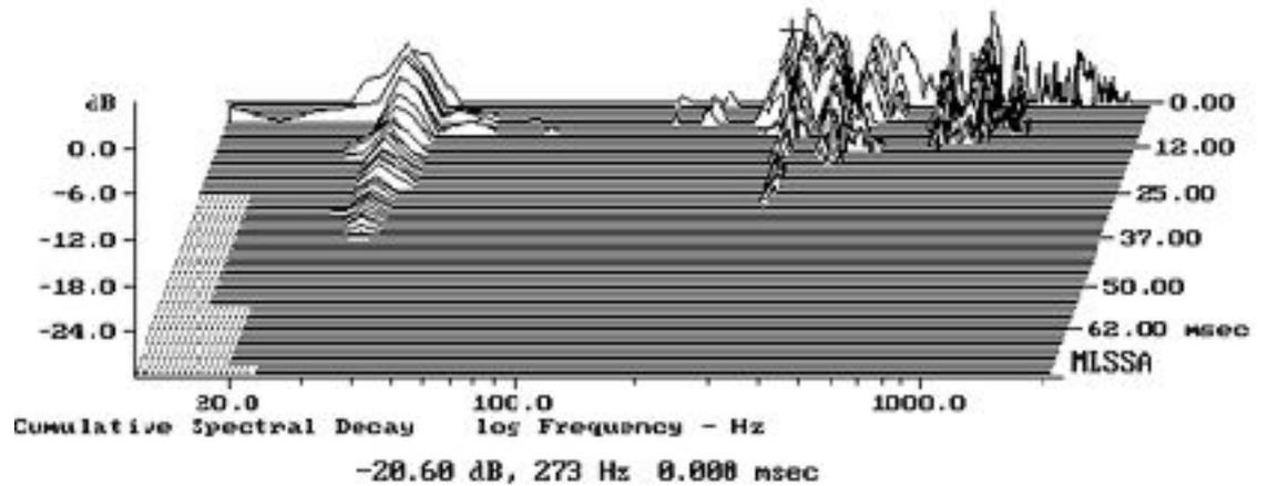
fastened to the cabinet's side panel 12" from base (MLS driving voltage to speaker, 7.55V; measurement bandwidth, 2kHz).
