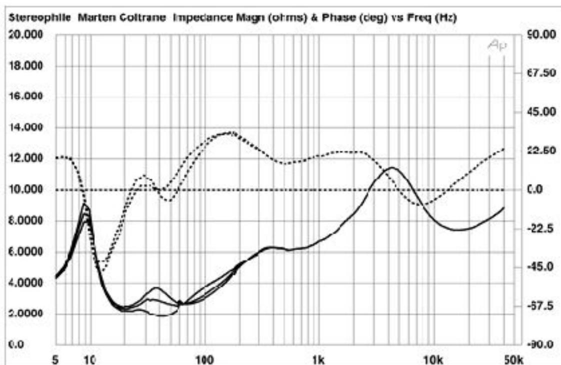
Fig.1 Mårten Design Coltrane, electrical impedance (solid) and phase (dashed) with rear-panel switch set to (from top to bottom at 40Hz): "5," "3," "0" (2 ohms/vertical div.).
