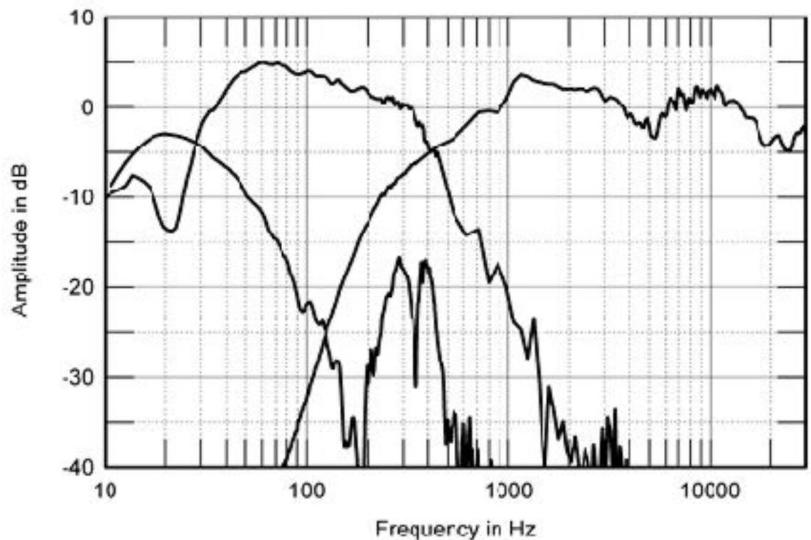
the nearest midrange, woofers, and port responses plotted below 350Hz, 440Hz, and 900Hz, respectively.
